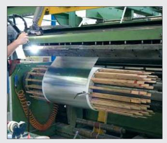
TIG welding in controlled atmosphere for LV connections.
