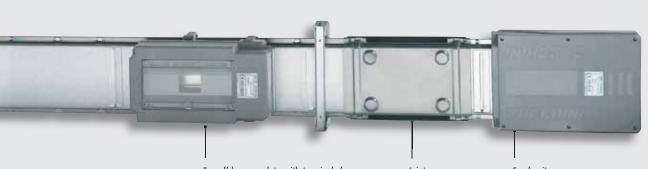
Tap-off box complete with terminals for cables of up to 25 mm². Made from self-extinguishing plastic material, ensures high mechanical resistance and resistance to static currents. Plug-in type boxes can be inserted and removed when the busbar is energized.
